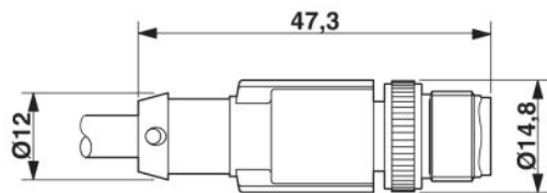
M12 x 1 male connector, straight, shielded
